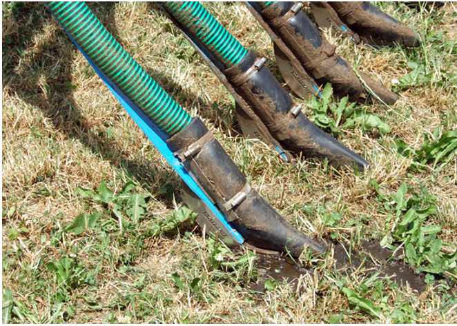
Fig. 15: Trailing shoe in details
