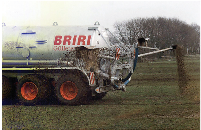
Fig. 18: Impact head distributor (with deflector plate)
